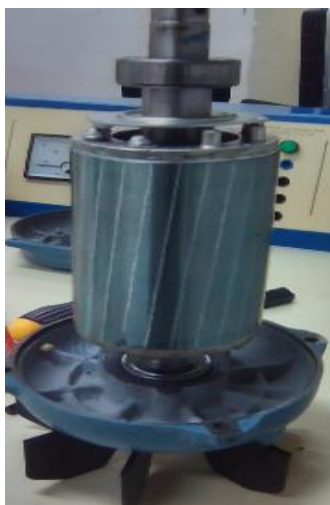
(a) Healthy rotor (without defect)
