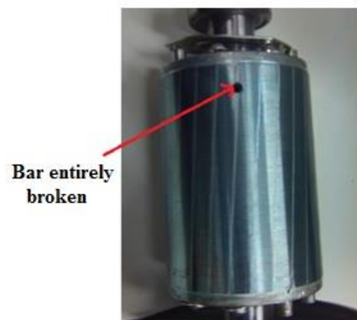
(b) Rotor at fault with a broken bar
