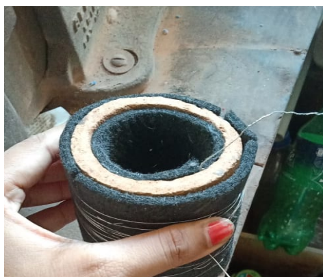
Figure 4 Electrodes wound around the membrane
