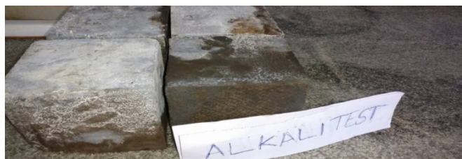
Figure 6. 28 days Alkaline cured concrete specimens
