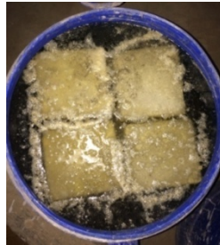
Figure4. Concrete Specimens under Acid Curing
