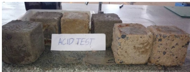
Figure5. 28 days acid cured concrete specimens
