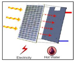
Figure1. Hybrid System Layout
