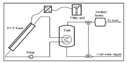
Figure2. Line Diagram of PVT System
