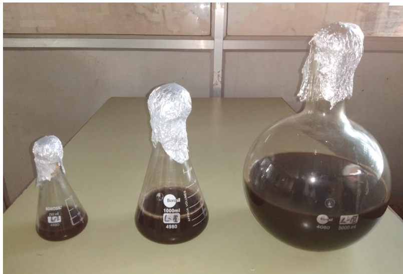
Figure III: Lab scale preparation of starter and batch culture.
