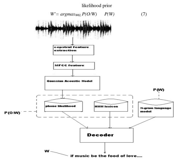
Figure 2: Architecture For Simplified Speech Recognizer Decoding Single Sentence.
