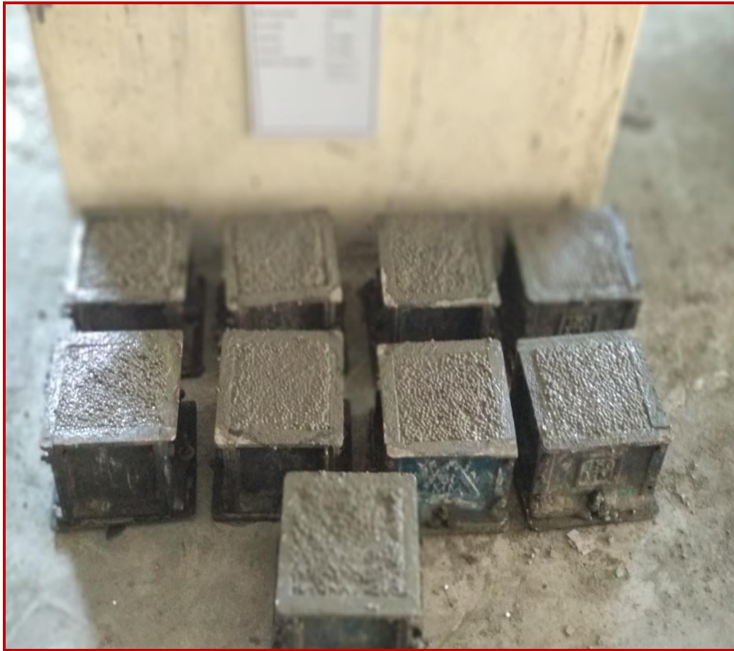
Fig.2.2 Casting of Specimen
