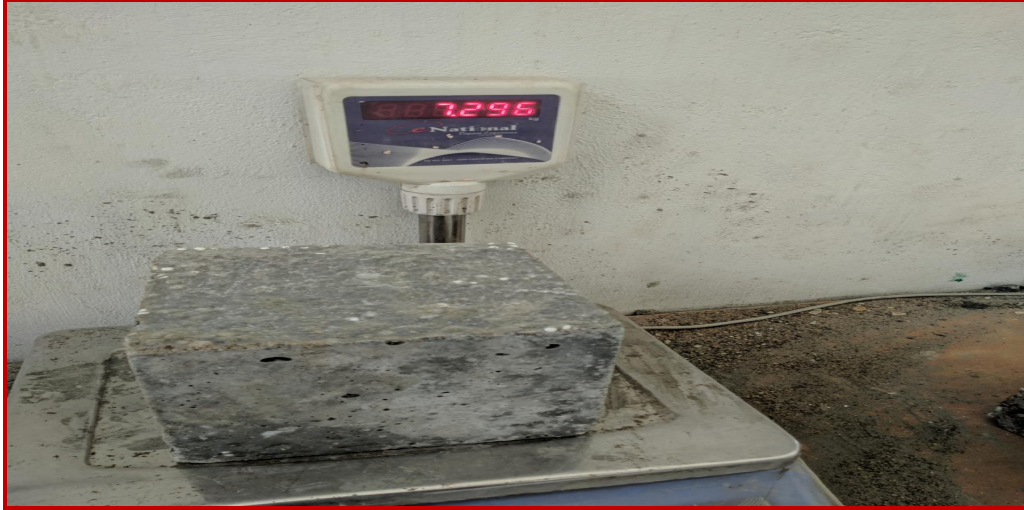
Fig.2.5 Weight of Eps Concrete Cube
