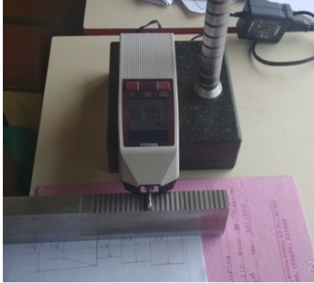
Figure 7 R_a measurement by using surface roughness tester
