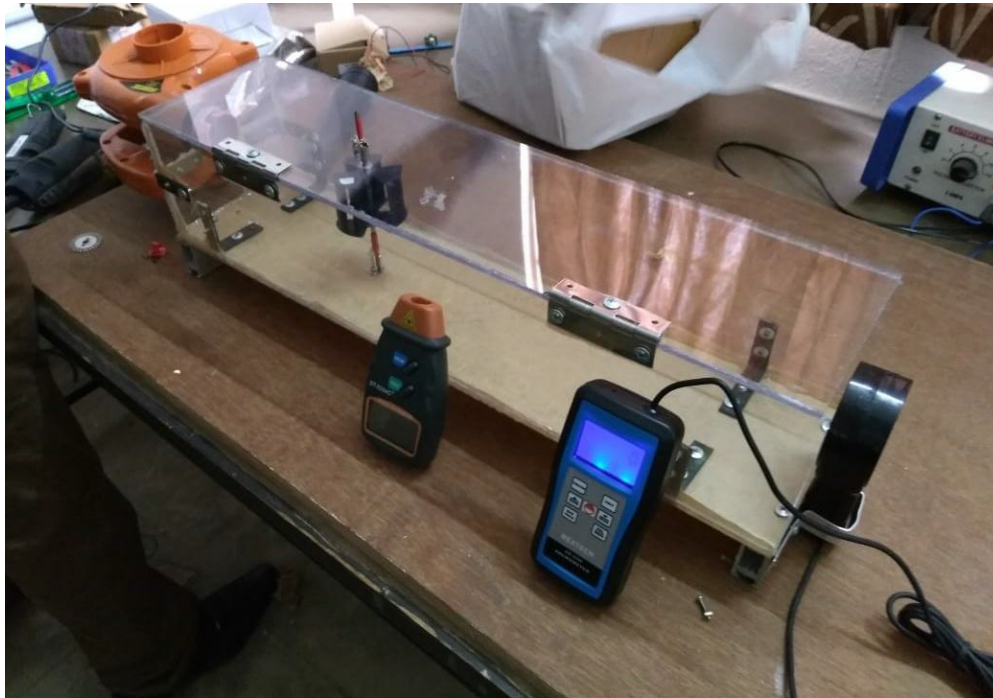
Fig. 5: Testing of Micro-Darrious vertical axis wind turbine
