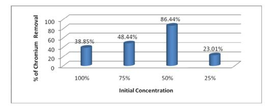
Fig: 4 Effect of Initial concentration of effluent using rice husk 5g/100ml at pH7.
