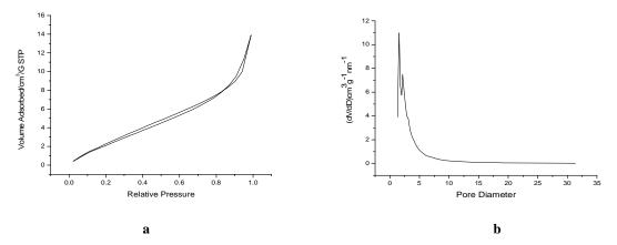
Fig 3: Bet surface area analysis. (a) adsorption desorption 77 K, (b) Pore volume distribution of rice husk
